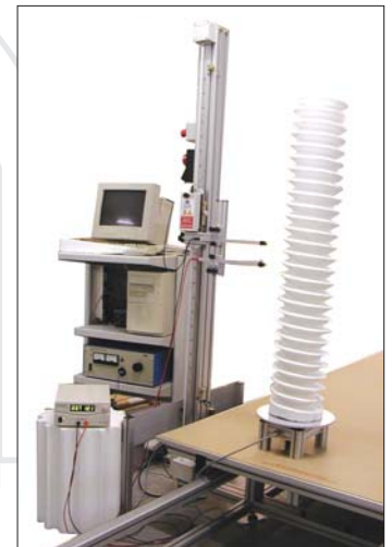
⊕ Turntable unit and form wire mounts for 3D working (e.g. producing spiral columns)
